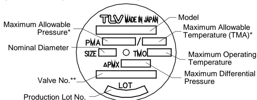
\* Maximum allowable pressure (PMA) and maximum allowable temperature (TMA) are **PRESSURE SHELL DESIGN CONDITIONS, NOT OPERATING CONDITIONS.**
