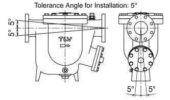
Make sure the product is installed with the raised TLV lettering on the body horizontal.
