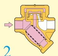
As temperature in the trap rises, the bimetal expands and releases the disc. The disc is forced downward by the low-pressure area created by the rapid flow of flashing condensate/steam below the disc, and the simultaneous high pressure in the pressure chamber above it. A steam jacket insulates the cap's pressure chamber from the radiant heat loss that could cause no-load actuation.
